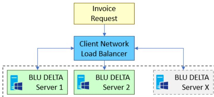
You can increase the invoice processing throughput and improve the reliability of the whole system by the usage of multiple BLU DELTA Servers. This works best in combination with a load balancer.
